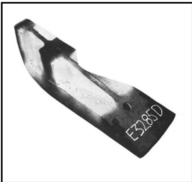
A low alloy steel casting containing surface crack indications (MPI)
