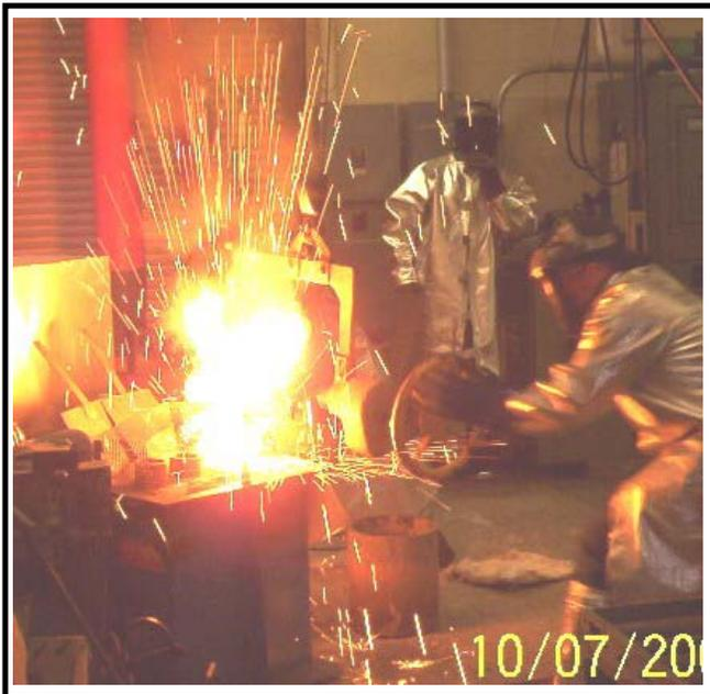
Students pouring lost foam castings with fill velocity data acquisition
